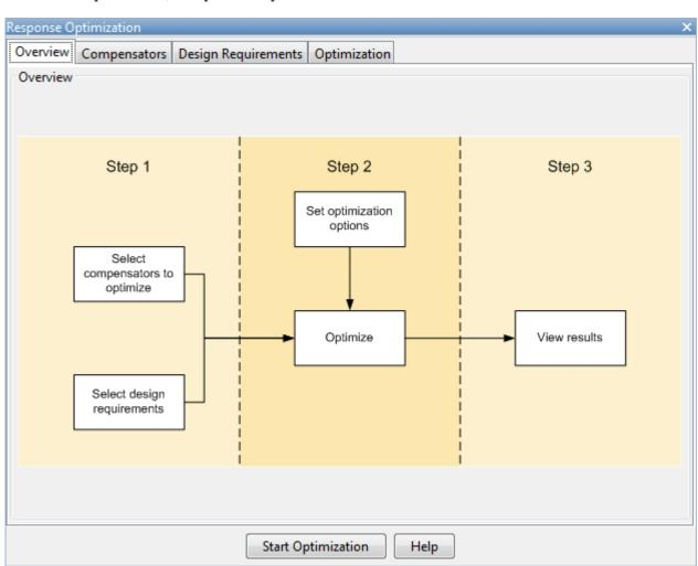
In the Response Optimization window, you can specify controller parameters and design requirements, and perform optimization.
