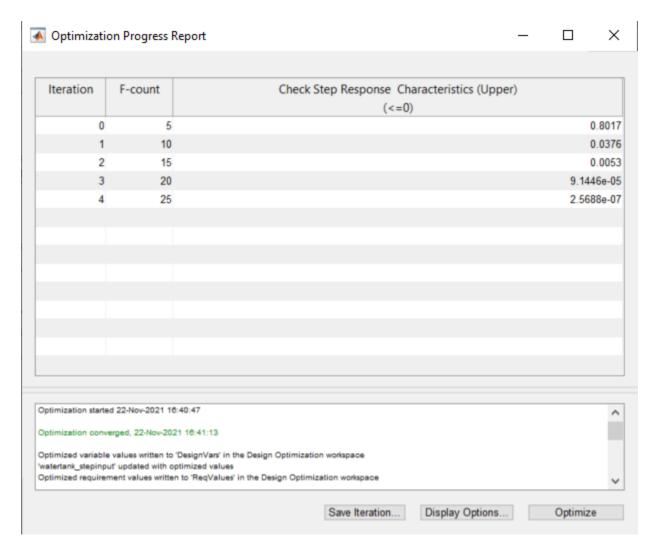
The message Optimization converged in the Optimization Progress Report indicates that the optimization solver found a solution that meets the design requirements within the tolerances and parameter bounds. For more information about the outputs displayed in the optimization, see "Iterative Display".
