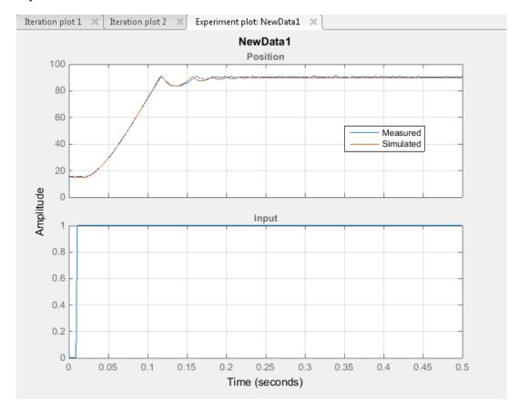
The data simulated using the estimated parameter values agree better with the measured data than when the parameter limits were not specified.
