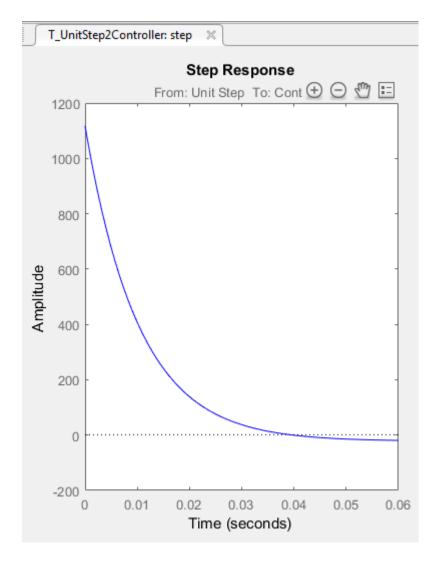
The plot shows that the peak value of the controller output is about 1100, which is large and can damage the plant. To limit the controller output, apply lower and upper bounds on the signal, as specified in "Design Requirements" on page 4-4.
