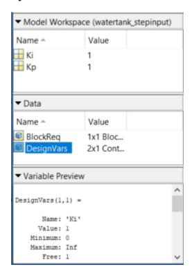
If your model has many parameters, you can first use sensitivity analysis to determine the most influential parameters to optimize, or to obtain initial guesses for the design variables. For more information, see "What is Sensitivity Analysis?" Using the **Sensitivity Analyzer** app, you can explore the response optimization design space by altering the design variables, identify the parameters that most influence the optimization problem, and compute initial values.
