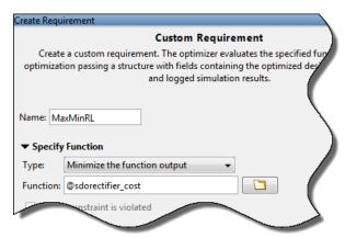
A new requirement variable MaxMinRL is created, and appears in the **Data** area in the **Response Optimizer**. The **Iteration plot 1** tab shows the value of MaxMinRL at each iteration during the optimization.
