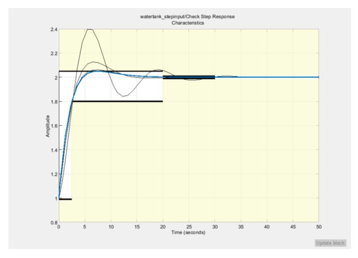
The plot displays the last five iterations. The final response using the optimized variable parameter appears as the thick blue line. The optimized response lies in the white region bounded by the design requirement line segments and thus meets the requirements.
