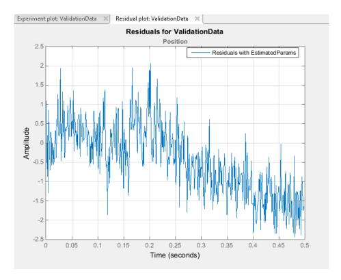
The difference between the simulated and measured data varies between 2 and -2.5. The residuals lie within 6% of the maximum output variation and do not display any systematic patterns. This indicates a good fit between the simulated output and measured data.
