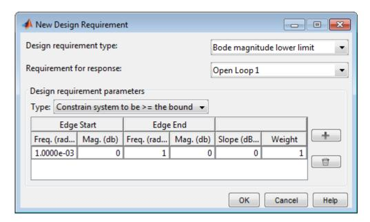
The Bode lower magnitude limit is added to the **Design requirements** tab.
