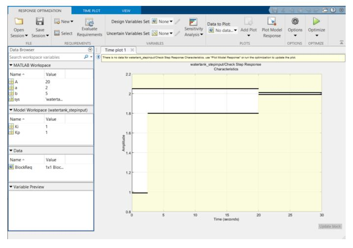
The region bounded by black line segments in **Time plot 1** shows the step response requirements that you specified in the Check Step Response Characteristics block.
